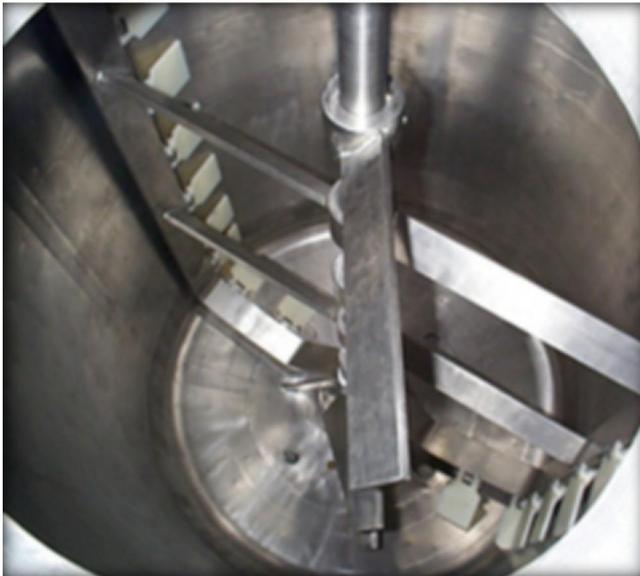
PerMix PCR series Contra Rotating Mixers have the advantage to combine the benefits of a turbine unit along with that of an anchor / scraper. PerMix PCR series Contra Rotating Mixers offer excellent mixing throughout the vessel as viscosities increase due to their double mix system. The wet end of PerMix PCR series Contra Rotating Mixers can be complete and installed into the tank prior to the vessel being completed or can be fully split to allow simple installation / removal.
