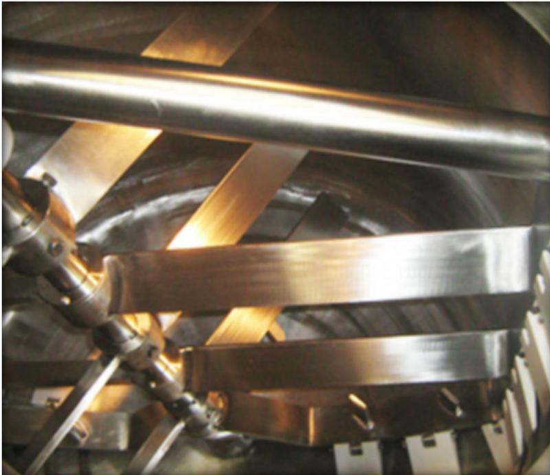
PerMix PCR series Contra Rotating Mixers are typically used when thick emulsions are produced by a bottom entry high shear emulsifier or homogenizer. They are also very useful for multi task vessels where different process duties are required. PerMix PCR series Contra Rotating Mixer is fitted with two drives: an anchor / scraper drive and a centrally mounted turbine drive. In effect it is two mixers joined together.
